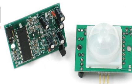
Fig 10. PIR Sensor & Pin details
