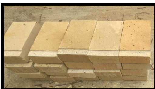
Figure 1.6. Hot face bricks IS 80
