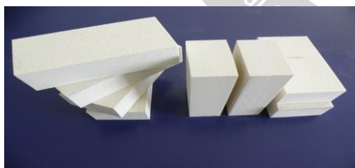
Figure 1.5. Cold Face bricks
