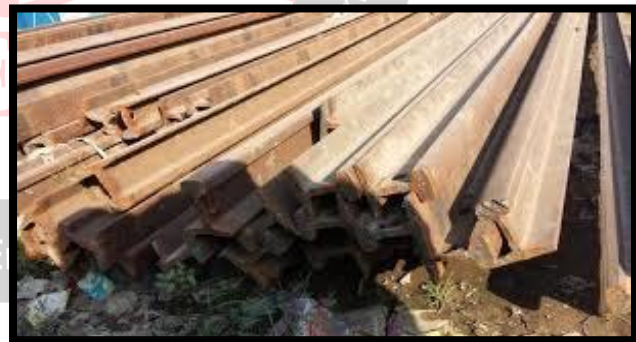
Fig1: Photograph of unused rail track due to corrosion problem
