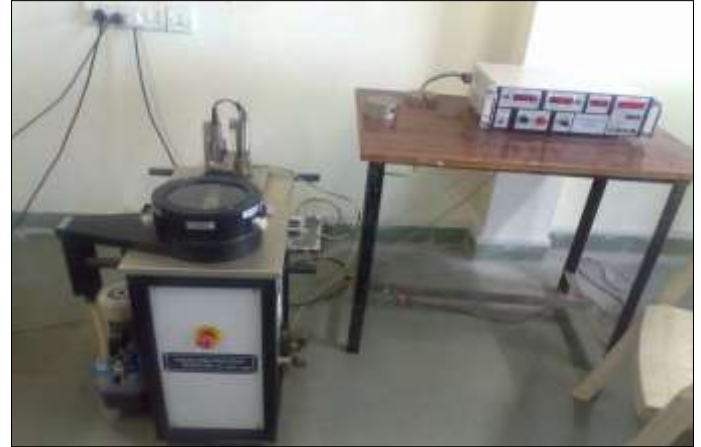
Fig.1 Photograph of experimental set up (Tribometer TR-20LE).
