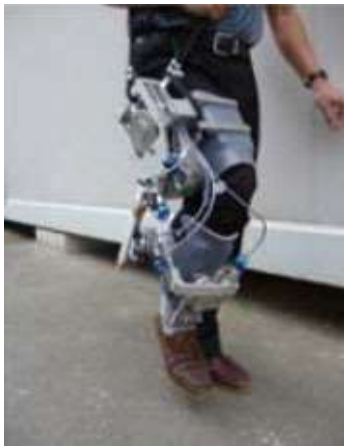
Fig 18 - Self-adjusting isostatic exoskeleton
