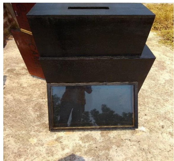
Fig. 3 Side View showing the flat plate collector
