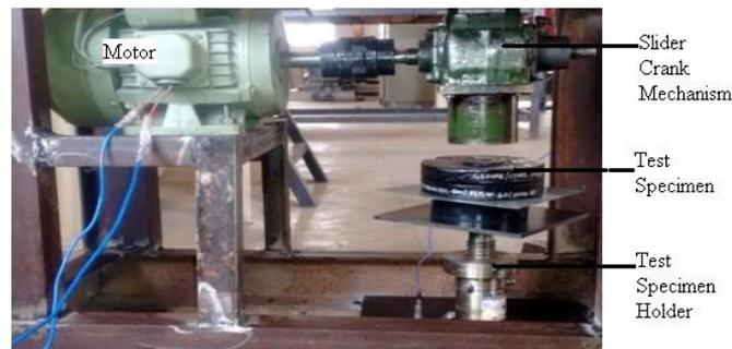
Fig 4: Vibration Test Rig
