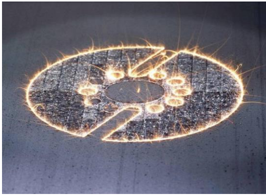
Fig 1.8: Selective laser sintering in action
