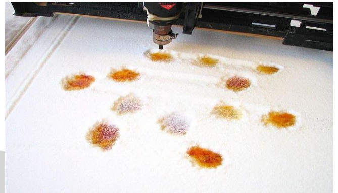
Fig 1.3: Granular Material Binding
