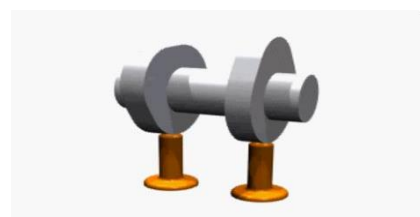
Figure 1.1 Computer animation of a camshaft operating valves
