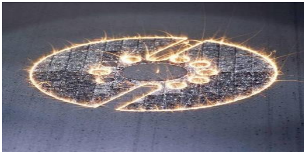
Fig 1.9: Selective laser melting in action
