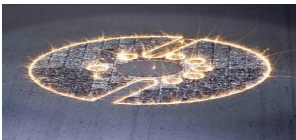
Selective laser sintering in action
