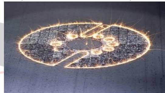
Fig 1.9: Selective laser melting in action
