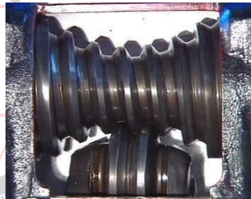
Fig.1.4 worm and roller
