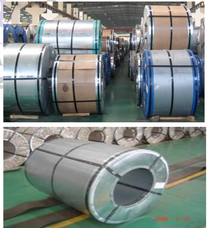
Fig 1. Sheet metal raw material in form of rectangular sheets and hollow cylindrical coils
