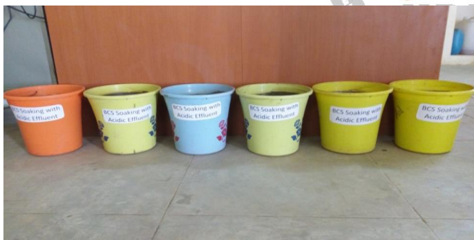
Photo 1 Storage of Black Cotton Soil treated (soaked) in Acidic effluent
