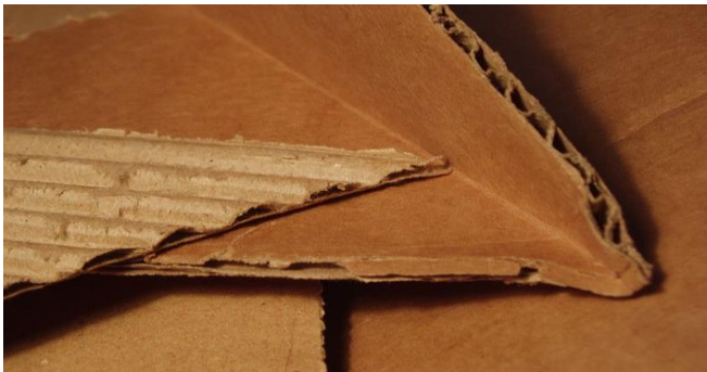
Fig. 5 shows the cross section of corrugated box. The air columns provide cushion and corrugations provide strength.
