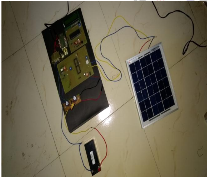
Fig.3: Design implementation of direct control method used in the MPPT.
