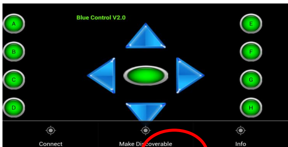
Fig. No.-4.2.6E Tap Connect to make the connection with HC-05
