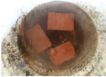
Fig 7 Water absorption test
