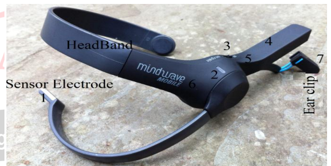
Fig.2 NeuroSky Mindwave Mobile EEG
