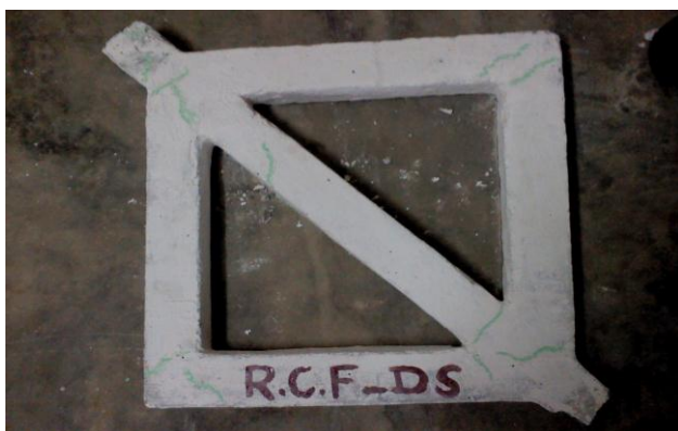
Fig. 9 Failure pattern of Frame with reinforcing band
