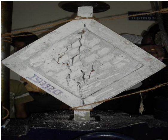
Fig. 8 Failure pattern of RC frame with infill
