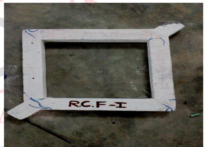
Fig. 6 Failure pattern of RC frame without infill
