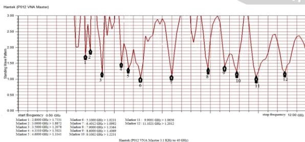
Fig.7 (d). Measured VSWR of the prototype crescent antenna
