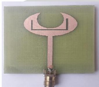
Fig.7 (a). Top view of Prototype Crescent-shaped antenna U slot
