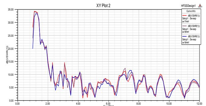
Fig.5 (b). Simulated VSWR for the proposed crescent antenna with variation in circular slot size and spiral slot in the ground plane
