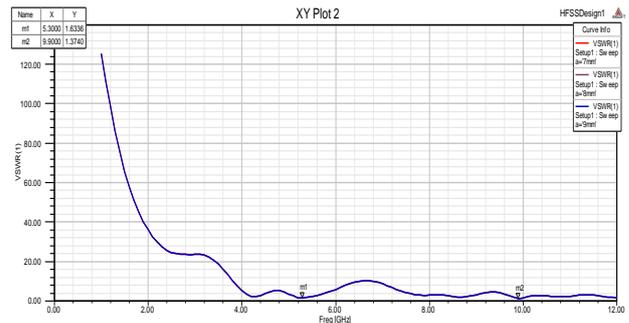
Fig.4 (b). Simulated VSWR for the full elliptical antenna
