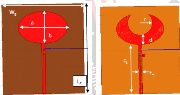
Fig.1. a) Full elliptical antenna b) Crescent antenna
