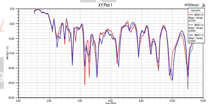
Fig.5 (a). Simulated return loss for the proposed crescent antenna with variation in circular slot size and spiral slot in the ground plane
