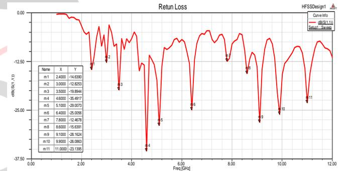
Fig.6 (a). Simulated return loss for the proposed crescent antenna with U slot
