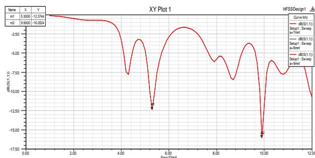
Fig.4 (a). Simulated return loss for the full elliptical antenna
