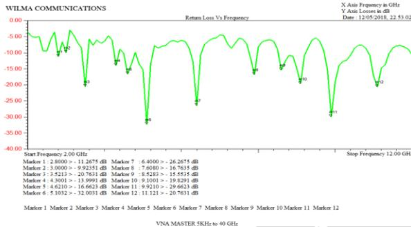
Fig.7 (c). Measured return loss of the prototype crescent antenna
