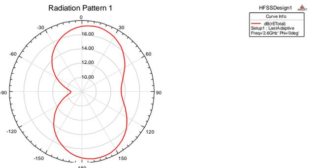
Fig.6(c). Simulated radiation pattern for Crescent antenna with U slot
