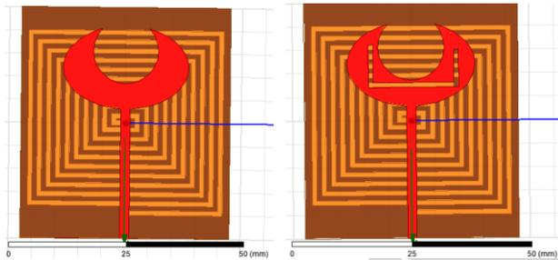
Fig. 3a. Crescent-shaped antenna with spiral ground plane. 3b. Crescent-shaped antenna with U slot in the patch
