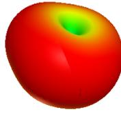
Fig. 6(d). Simulated gain for Crescent antenna with U slot
