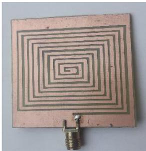
Fig.7 (a). Bottom view of Prototype Crescent-shaped antenna with spiral ground plane.
