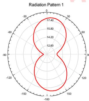
Fig. 5(e) Simulated radiation patterns for Crescent antenna
