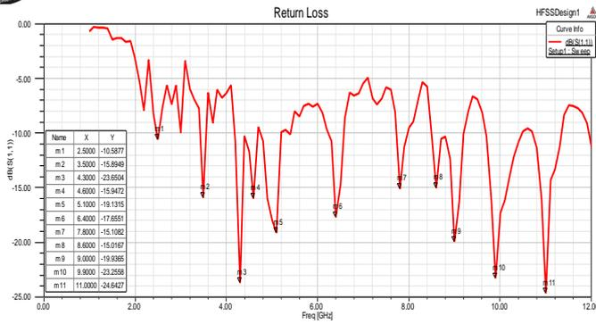
Fig.5(c). Simulated returns loss for the proposed crescent antenna with 7mm circular slot and spiral slot in the ground plane
