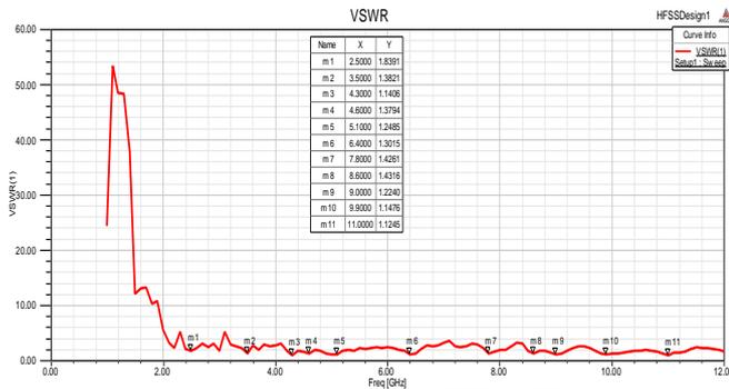
Fig.5 (d). Simulated VSWR for the proposed crescent antenna with 7mm circular slot and spiral slot in the ground plane
