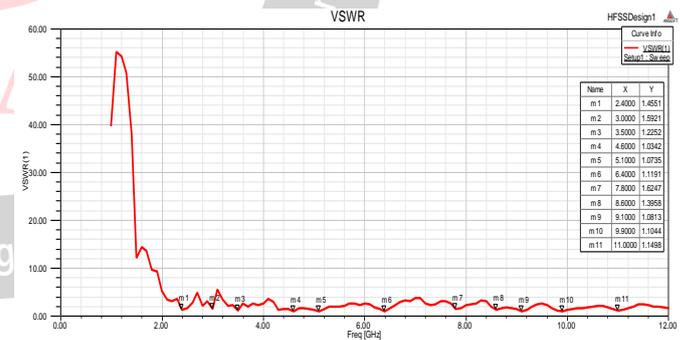
Fig.6 (b). Simulated VSWR for the proposed crescent antenna with U slot
