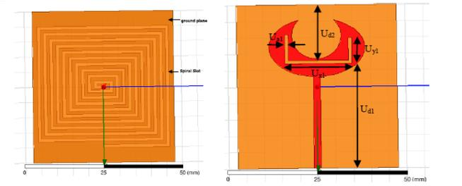
Fig.2a. One arm spiral ground slot 2b. Crescent Antenna U slot
