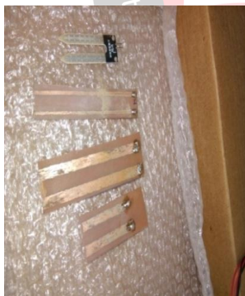
Fig. 2 (a): Resistive soil moisture sensors of different dimensions
