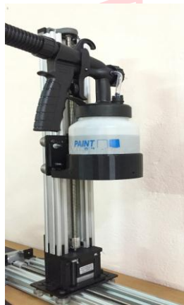
Fig. 8. Y axis with spray painter attached
