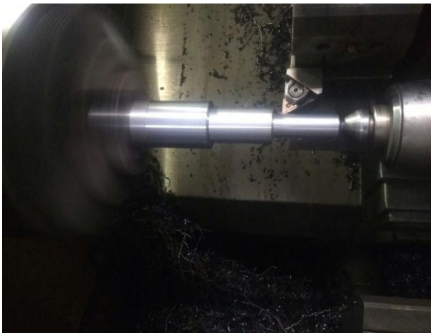
Figure 3. Step turning work piece
