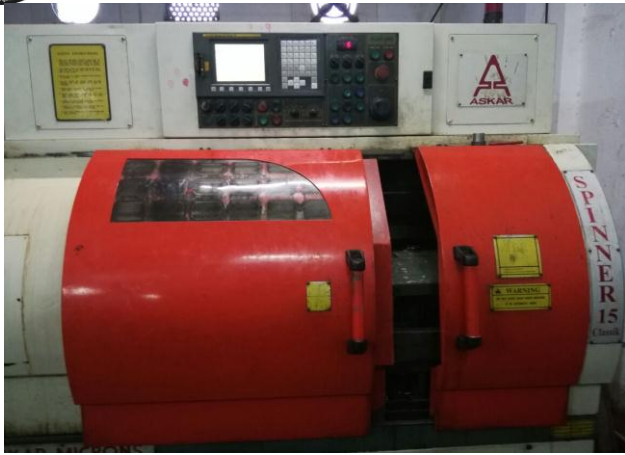
Figure.2 Spinner CLASSIK CNC Lathe machine
