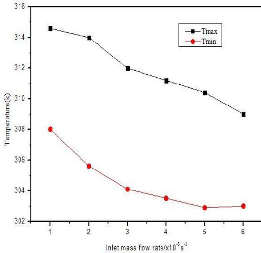
Fig 4. Temperature of the module under different inlet mass flow rates.
