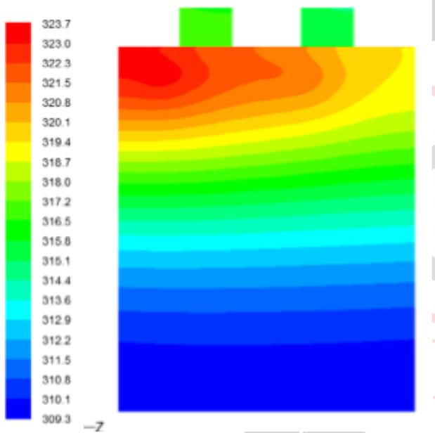
Fig 2. Temperature distribution of lithium ion battery at end of 2c discharging
