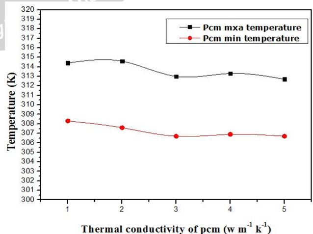
Fig.6 Temperature of the module under different thermal conductivity of PCM.
