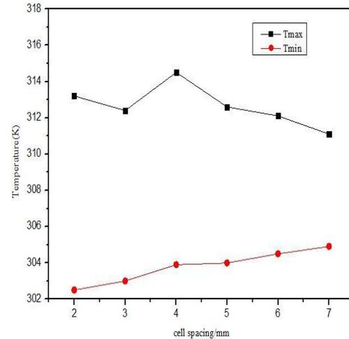
Fig.3(a) Temperature of the module under different space between adjacent batteries
