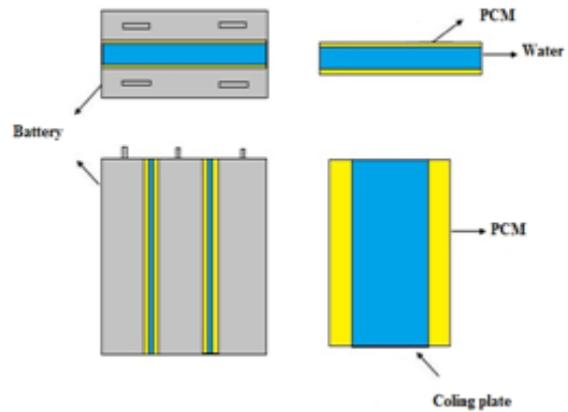
Fig.1.Schematic of lithium ion battery module with PCM /water cooling plate.
