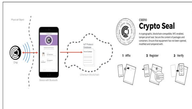
Fig. No. 2: Chroniled asset tracking blockchain concept showing single application Crypto Seal
