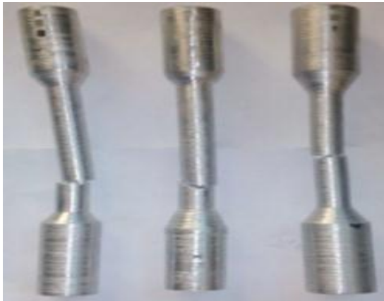
Fig. 2 Specimen after tensile test
