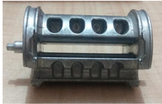
Figure 21: As cast of Cylinder shell produced from HPDC method
