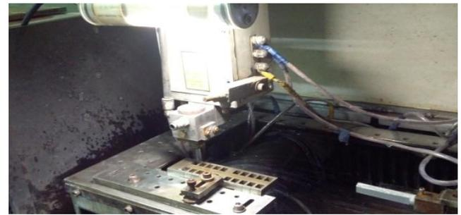
Fig 1: Experimental setup of WEDDM
