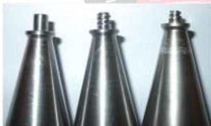
Fig. 1. FSW tools with a) Cylindrical Unthreaded, b) Cylindrical threaded and c) Conical Threaded profile [27]
