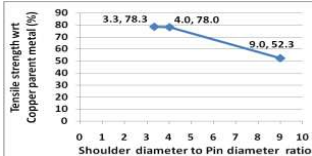
Figure 7. Graph of Tensile strength achieved with respect to copper parent metal vs. SPR [13,14,30]
