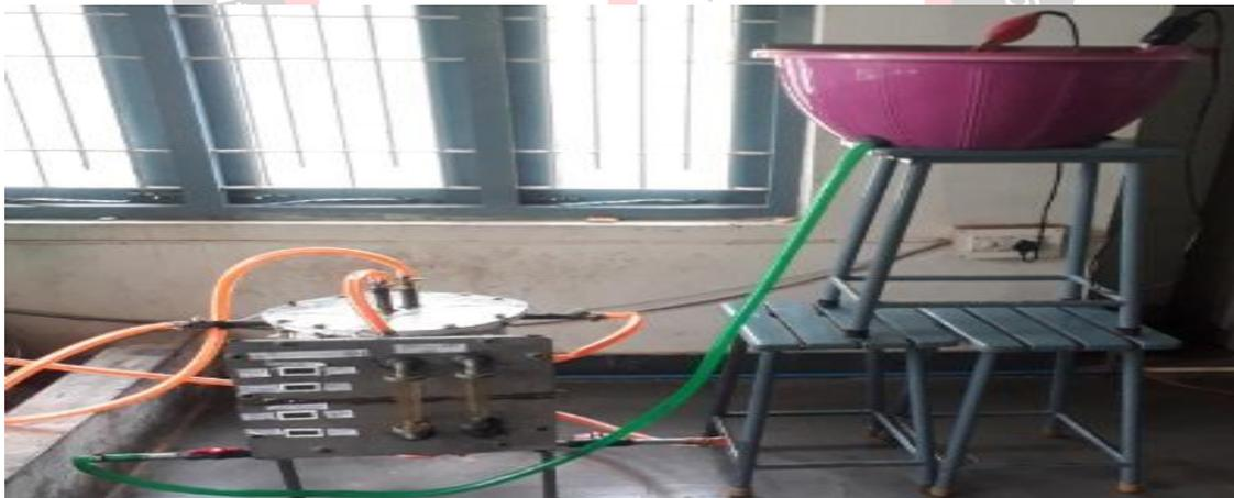
Fig 1 Experimental setup of spiral plate heat exchanger.
