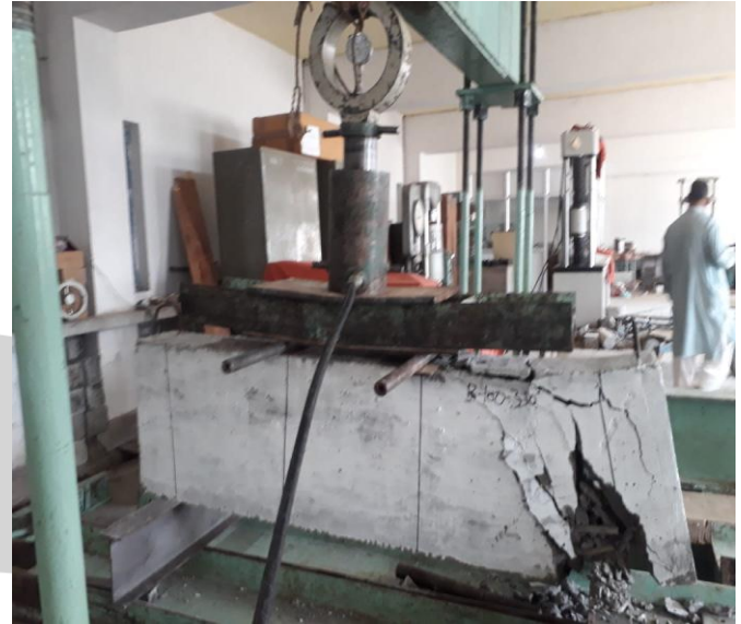
Figure 6: Shear failure of Deep beam
