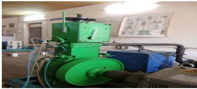
Figure.1, Computerized VCR Engine Test Rig
