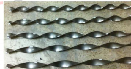
Fig.5 Twisted tape separated from tube wall
