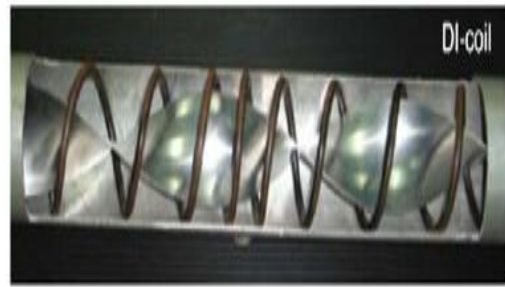
Fig.10 Non uniform wire coiled with twisted tape
