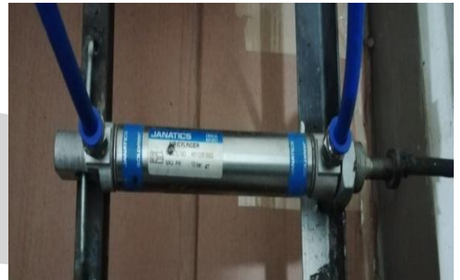
Fig 3:-Single-Acting Pneumatic Cylinder
