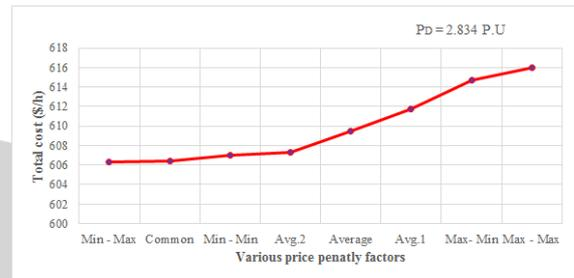
Fig. 4 Total cost versus various price penalty factors of IEEE 30 bus system with valve point with loss
