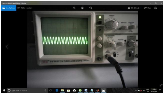
Fig 13: FIR filter output for input signal frequency=2000Hz
