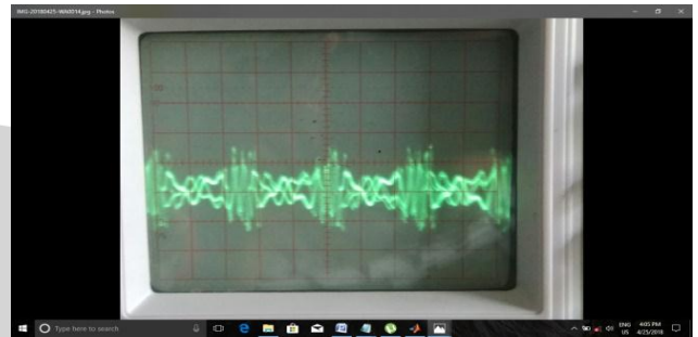
Fig 17: IIR filter output for input signal frequency= 4KHz
