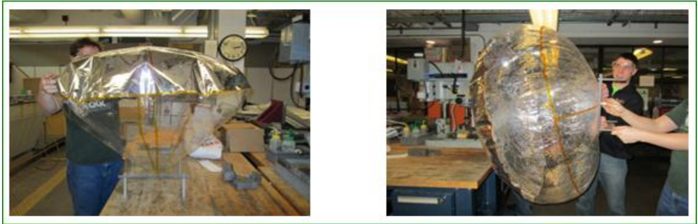
Fig. 2. Conical and cylindrical configurations of Inflatable antenna [4]
