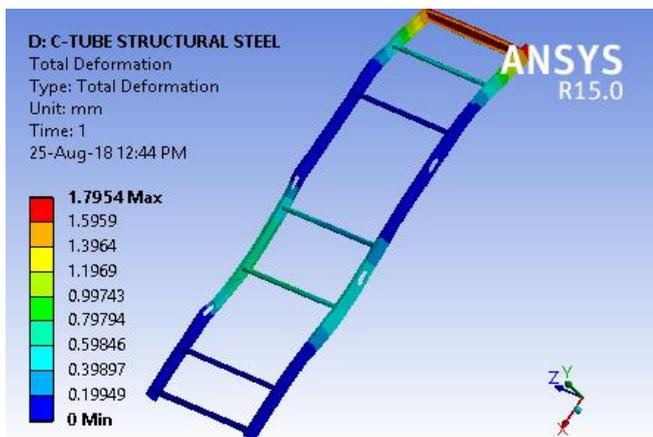
Fig 23: Deformation
