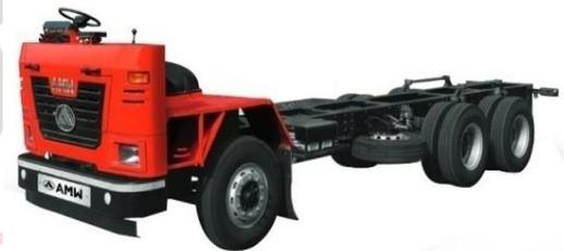
**Fig 1: Ladder type chassis**
