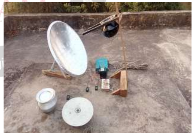
Fig 2: Experimental setup for evaluating the performance of parabolic dish collector system
