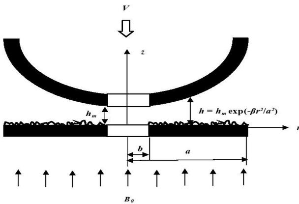
**Figure 1: Pictorial presentation of rough curved annular plates.**
