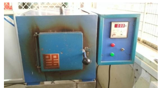
Figure 2c Muffle furnace is used for sintering
