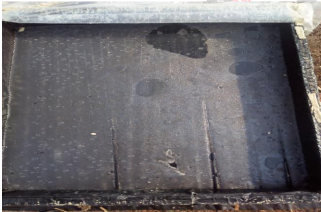
Figure 11: Surface solidification of paraffin wax due to outflow from the aluminum tube.
