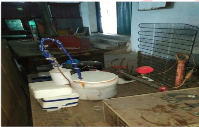
(b) Actual Setup of the vapour compression refrigeration system with an ejector and secondary evaporator
