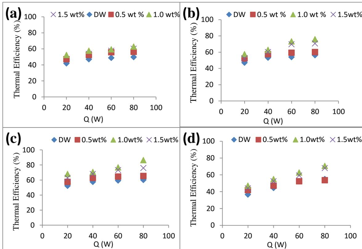
Fig.5 Thermal efficiency of heat pipes at various inclination angles ( $\theta$ ): (a)  $0^\circ$  (b)  $30^\circ$  (c)  $60^\circ$  (d)  $90^\circ$
