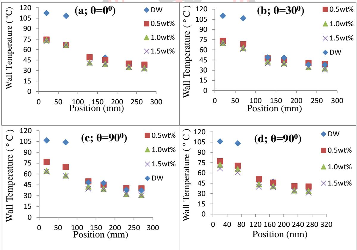
Figure.4 (a-d) Distribution of wall temperature at different tilt angle for 80W
