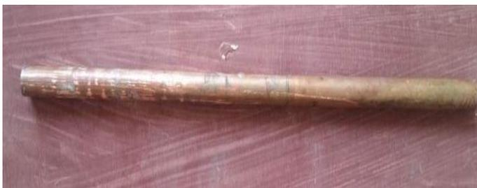
**Fig.2 Sintered wick heat pipe used in experiment**
