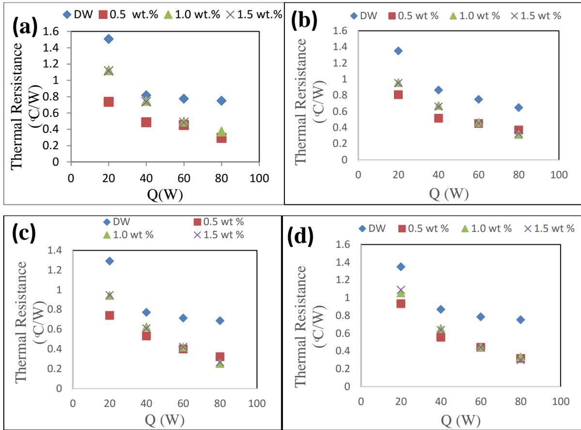
Fig.6 Thermal resistance of heat pipes at various inclination angles (θ): (a) 0° (b) 30° (c) 60° (d) 90°
