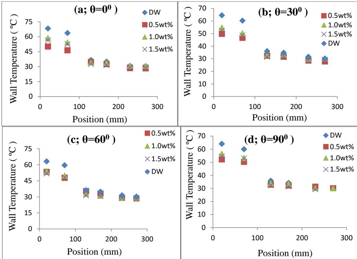
Fig.3 (a-d) Distribution of wall temperature at various tilt angles for 20W
