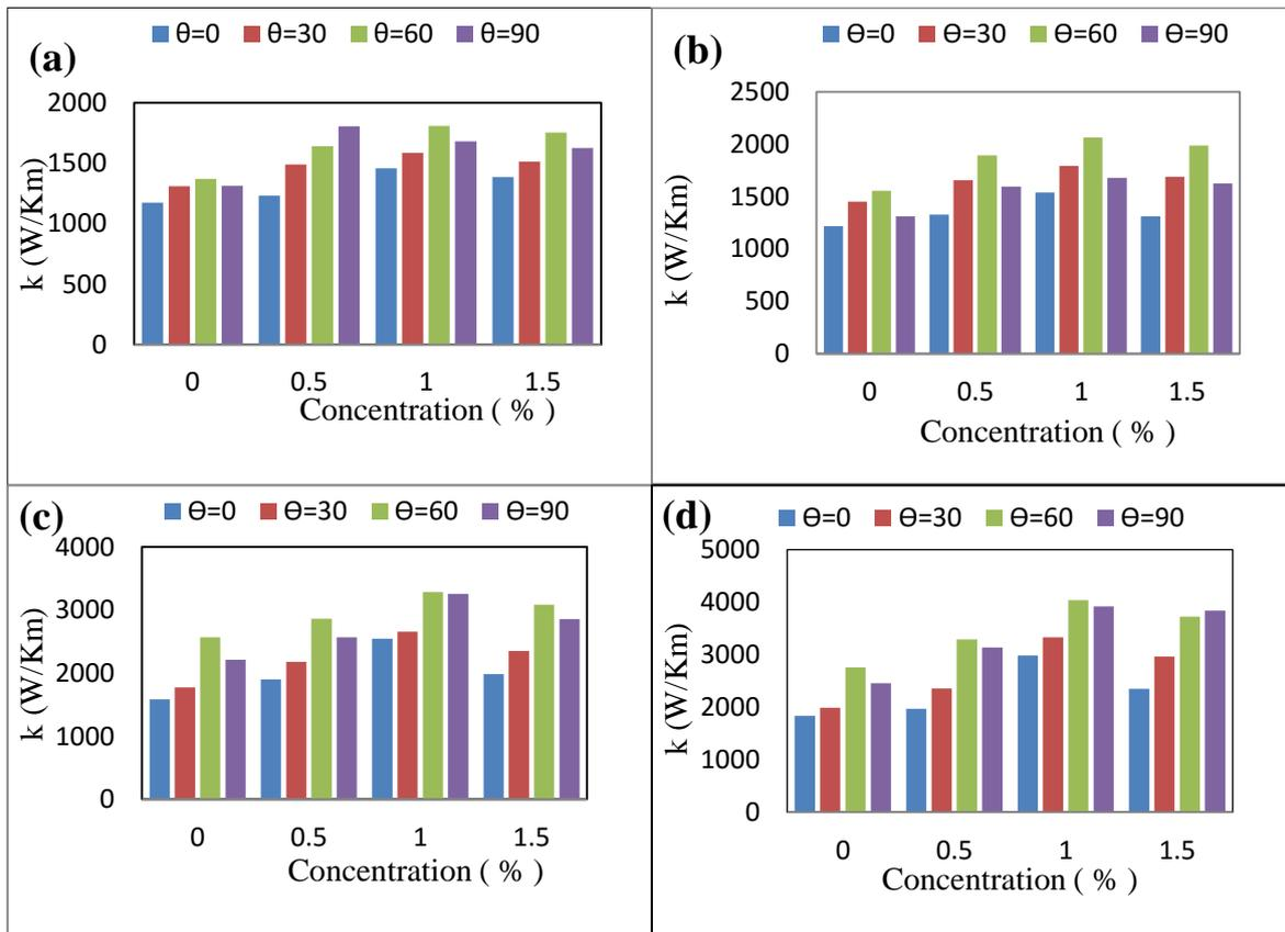
Fig.7 Effective thermal conductivity of heat pipes (sintered wick) for different heat input rates: (a) 20 W, (b) 40 W, (c) 60 W, (d) 80 W.
