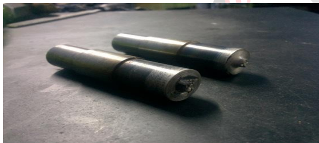
Figure 2 shows FSP tool of different profiles.
