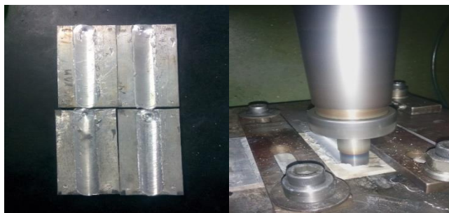
Figure 3a & 3b shows FSPed plates and processing procedure.
