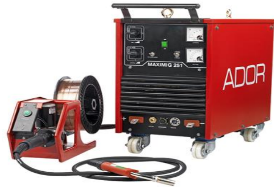
Fig 1: MAXIMIG 251 CD MIG welding machine (Courtesy: Production Workshop, B.I.T Mesra, Ranchi)
