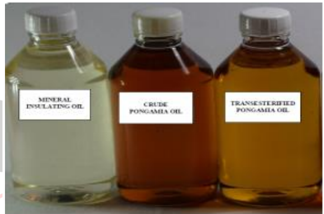
Fig.6. Samples of mineral oil and pongamia oil
